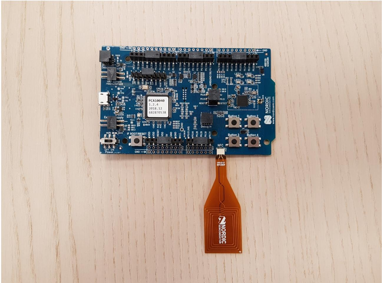
*NFC tag used as a prototype for system operation*
